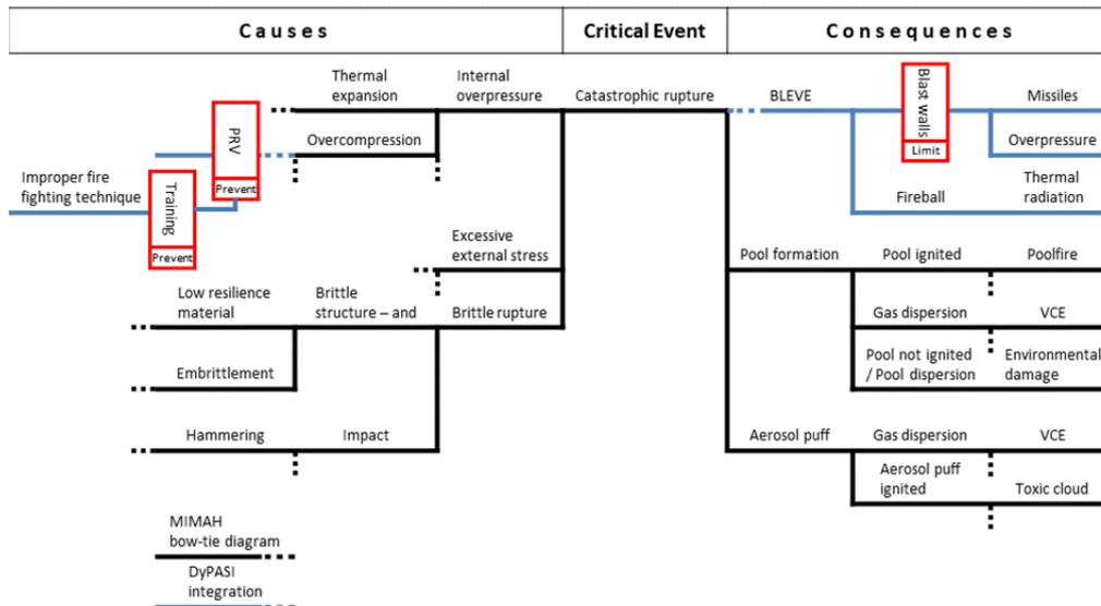
Figure 2: Bow-tie diagram updated with the DyPASI integrations (light blue dotted line) adapted from (Paltrinieri et al., 2015). Safety barriers in red boxes to avoid the critical event or to limit the consequences
