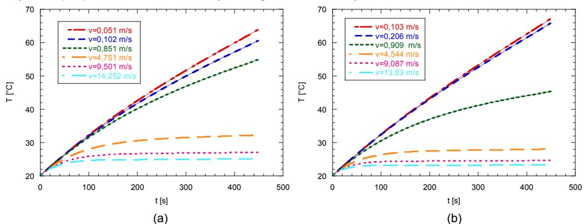
Figure 4 Temperature trends at a discharge rate of 20 A,  $d= 1\text{mm}$ ,  $T_a=20^\circ\text{C}$ : a) Midel ICE, b) GaldenHT135.
