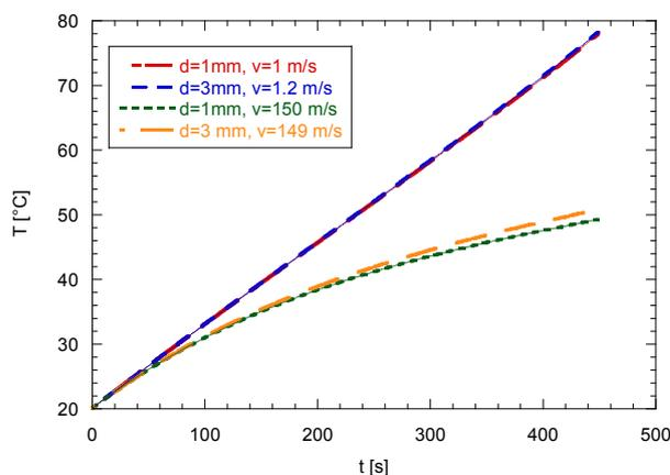
Figure 3 Temperature trends for cylindrical cells discharged with a current of 20 A and cooled with air at the minimum and maximum pumping powers. Distances between the cells:  $d=1\text{mm}$  and  $d=3\text{mm}$ ,  $T_a=20^\circ\text{C}$ .
