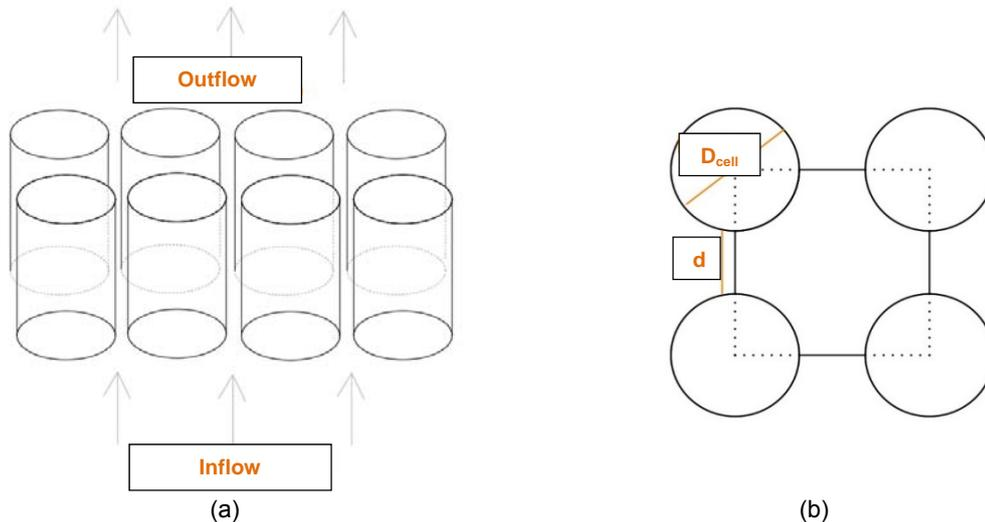
Figure 1 Flow direction a) and passing area b) of the cooling fluid.
