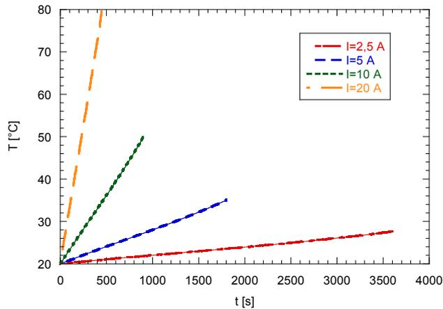
Figure 2 Comparison between the temperature trends of cylindrical cell, at different discharge rates, using air in free convection,  $T_a=20^\circ\text{C}$ ,  $d=1\text{mm}$ .
