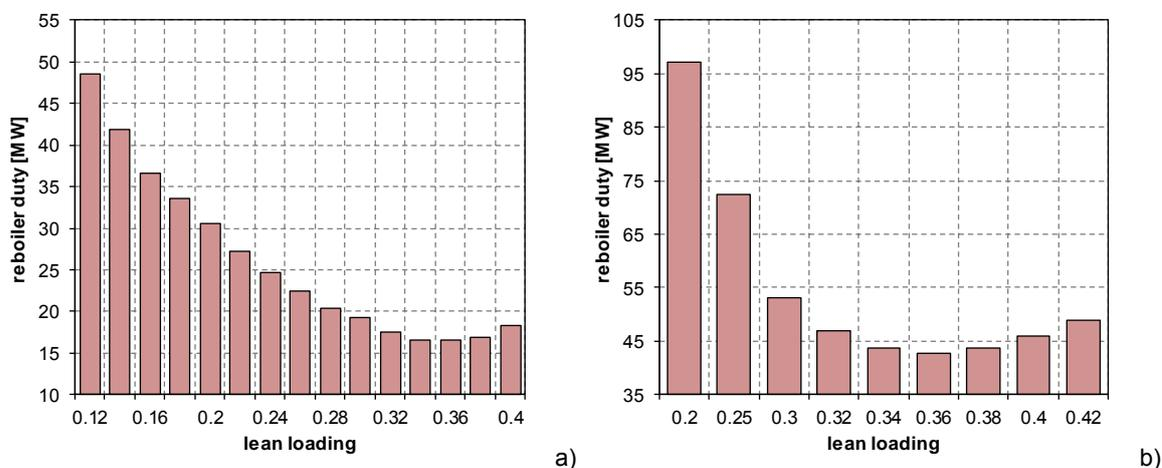
Figure 2: Variation of reboiler duty (expressed in thermal MW) referring to the *CO<sub>2</sub>* removal in one single absorption column with lean loading for a) scheme with 40 parallel absorption tray columns and b) scheme with 20 parallel absorption tray columns.
