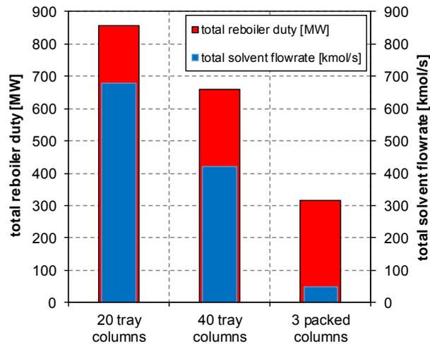
Figure 4: Total reboiler duty (expressed in thermal MW) and total solvent flowrate for the three schemes.
