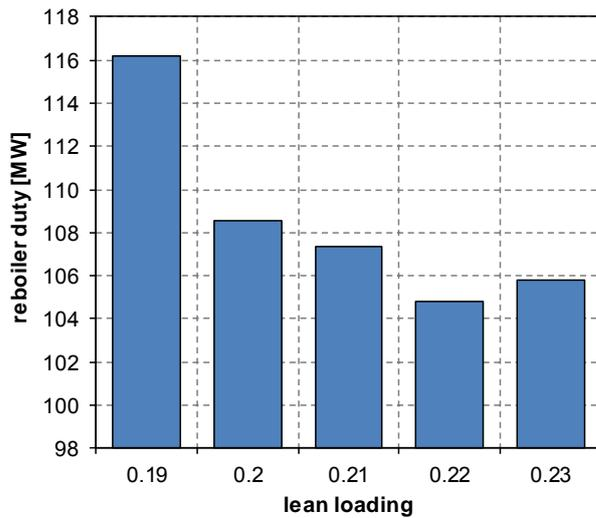
Figure 3: Variation of reboiler duty (expressed in thermal MW) with lean loading (mol CO<sub>2</sub>/mol MEA) for the scheme with 3 parallel packed columns.
