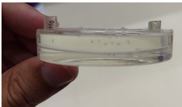
Figure 1. Microfluidic device for in-situ analysis of water / ethanol and oil / ethanol using Raman Spectroscopy.
