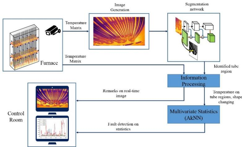
Figure 3: The overall monitoring framework for both shape and temperature monitoring.
