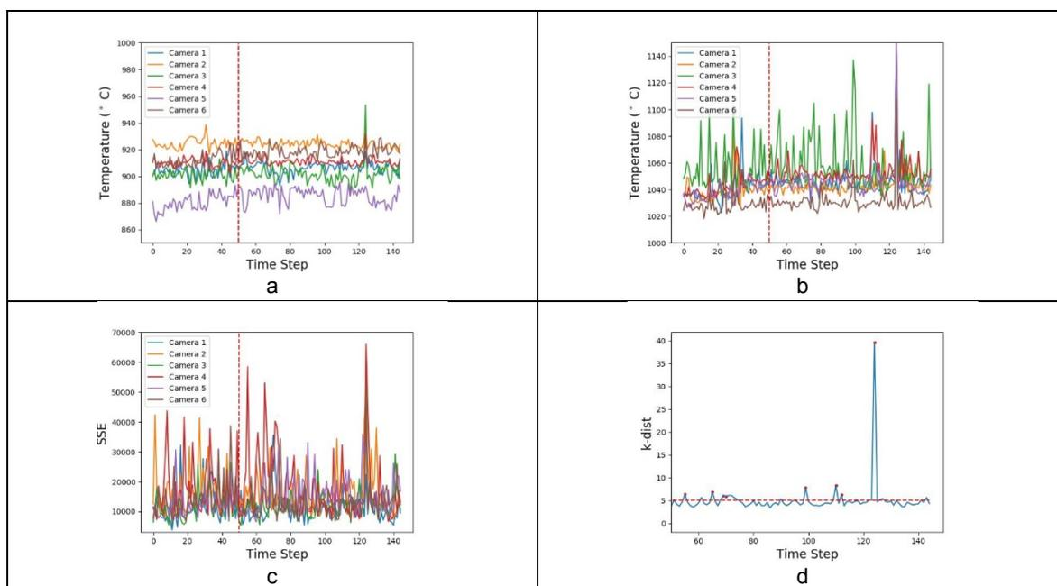
Figure 5: Monitoring results from the proposed framework. (a) Averaged tube temperature. (b) Maximum tube temperature. (c) SSE for shape monitoring. (d) Fault detection results from the AkNN method. The first 50 data samples are used to train the AkNN method, while the rest 100 are testing samples.
