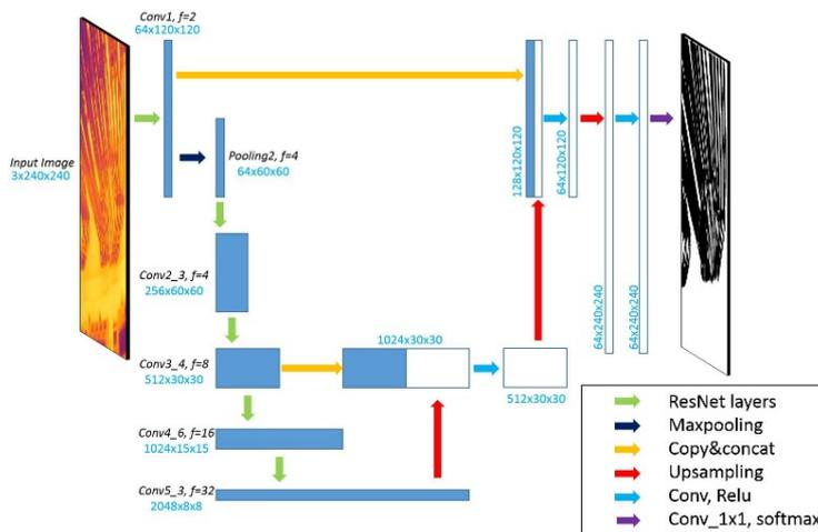
Figure 2: The proposed infrared photo segmentation network
