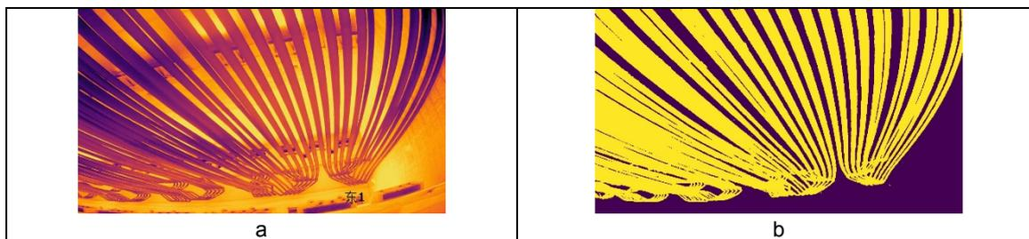
Figure 4: A demonstration of the segmentation results. (a) The raw infrared photos. (b) The segmentation results. The tube area is colored in yellow and the background is colored in purple.
