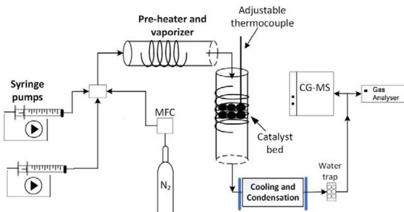
Figure 1: Experimental set-up
