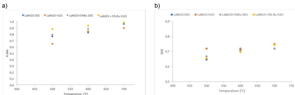
Figure 4: a) Carbon conversion as a function of temperature with the prepared catalysts of ABE, b) H<sub>2</sub> selectivity
