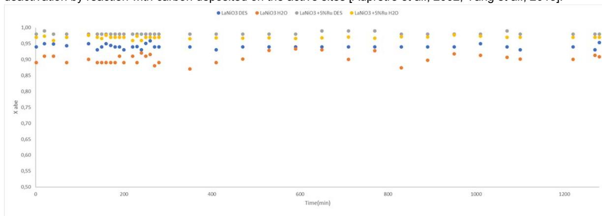
Figure 5: Conversion of ABE in the long duration tests for the four catalysts at 700 °C.
