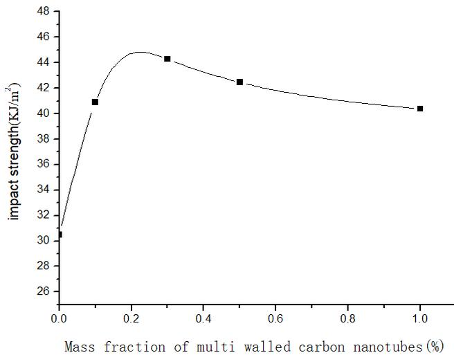
Figure 3: Impact strength of composite under different content CNTS
