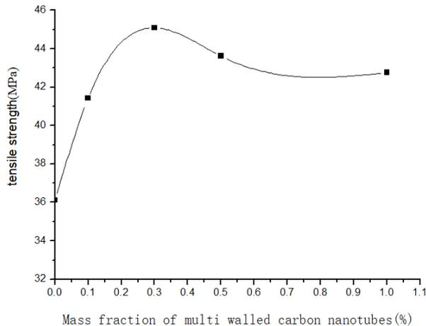
Figure 1: Tensile strength of composite under different content CNTS
