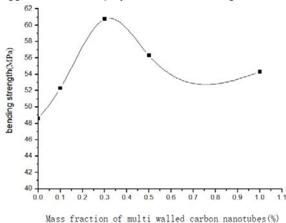
Figure 2: Bending strength of composite under different content MWNTS
