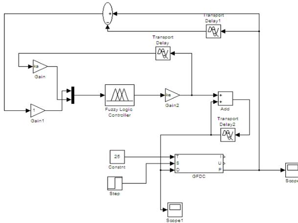
Figure 6: MPPT system simulation model in Matlab/Simulink environment
