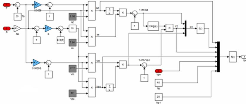
Figure 2: Photovoltaic cell simulation model
