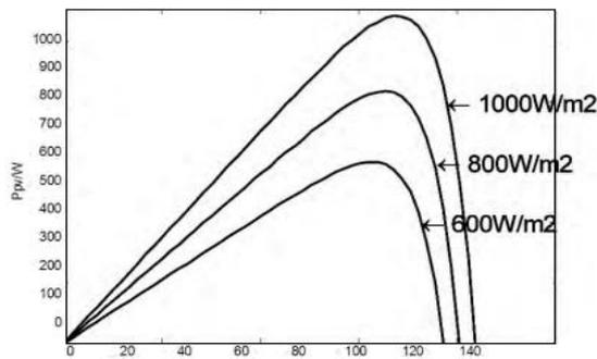
Figure 3: P-V curve when S changes
