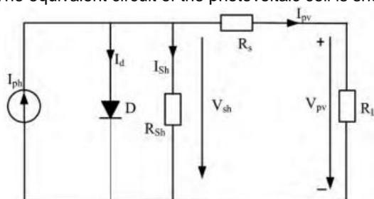
Figure 1: Equivalent circuit of the photovoltaic cell model
