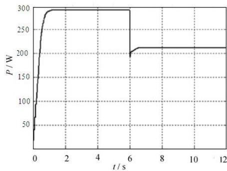
Figure 8: Conversion waveform of output power when the light intensity decreases
