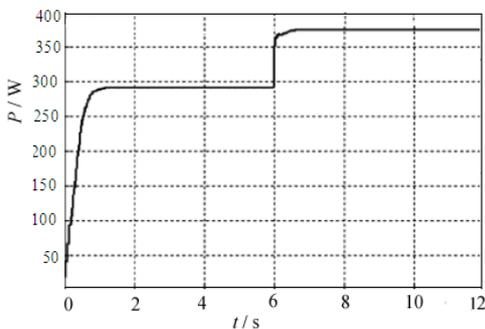
Figure 7: Conversion waveform of output power when the light intensity increases
