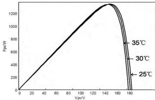
Figure 4: P-V curve when T changes
