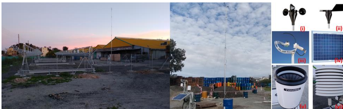
Figure 2: (a) Solar PTC system (b) Weather station (i) anemometer (ii) Wind direction vane (iii) Irradiometer (iv) PV-panel (v) rain gauge (vi) Temperature & RH probe
