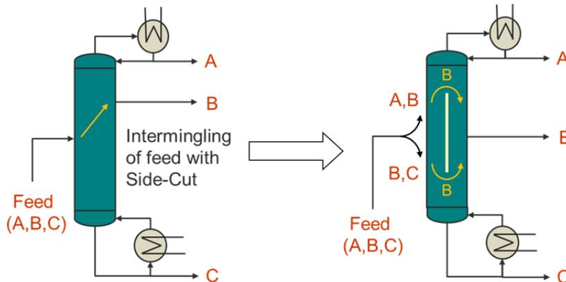
Figure 3: Conventional Side-Cut Column v/s Proprietary DWC
