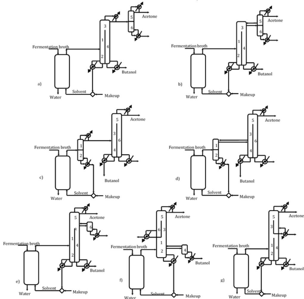
Figure 3. Liquid-liquid extraction assisted non-conventional DWC configurations
