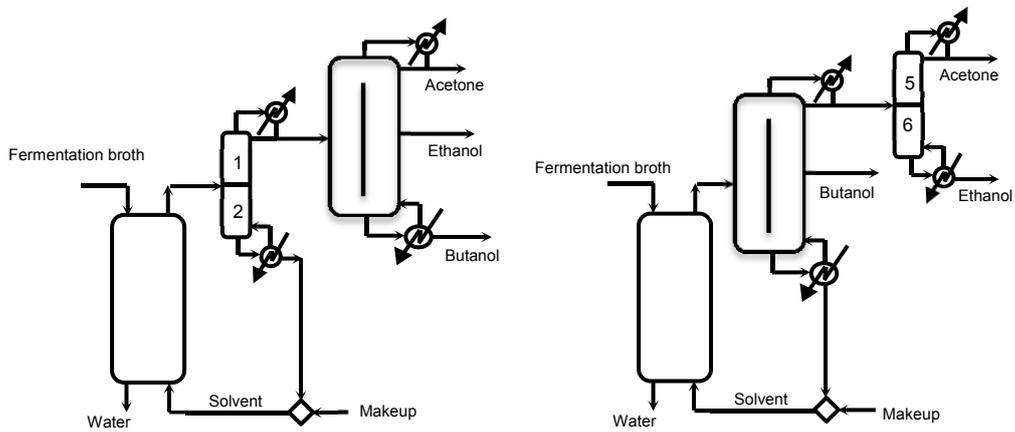
Figure 2. Liquid-liquid extraction assisted conventional DWC configurations
