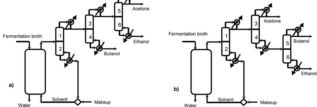
Figure 1 Liquid-liquid extraction assisted simple columns: (a) indirect sequence (HLL-ISC), (b) indirect-direct sequence (HLL-IDSC)
