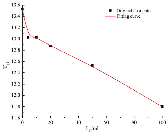
Figure 7: Response time constant  $T_{P1}$  varies with gas sampling volume  $L_0$
