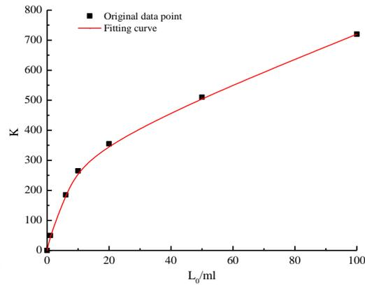
Figure 6: Response stability amplitude  $K$  varies with gas sampling volume  $L_0$
