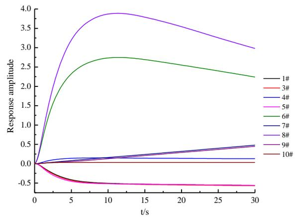
Figure 9: Response curve of e-nose gas sensor array to diesel oil gas
