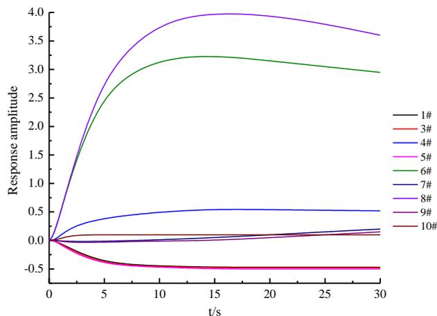
Figure 10: Response curve of diesel/gear oil mixed gas for e-nose gas sensor array
