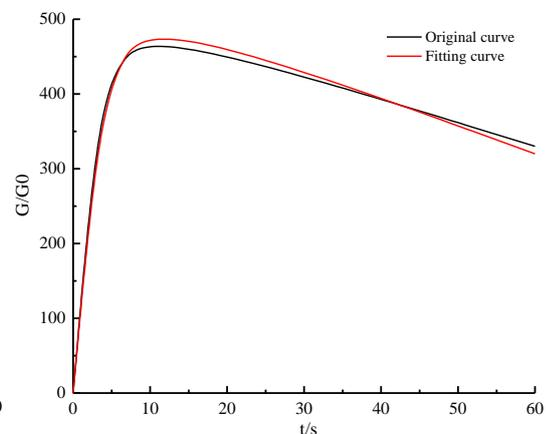
Figure 4: Comparison of the sensor response fitting results with the actual response
