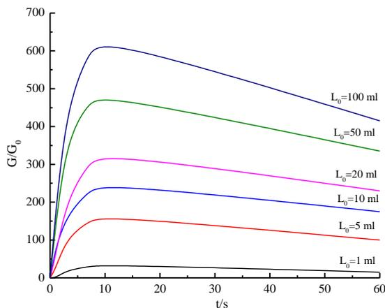
Figure 3: 2# sensor response curve of different concentrations of diesel oil volatile gas
