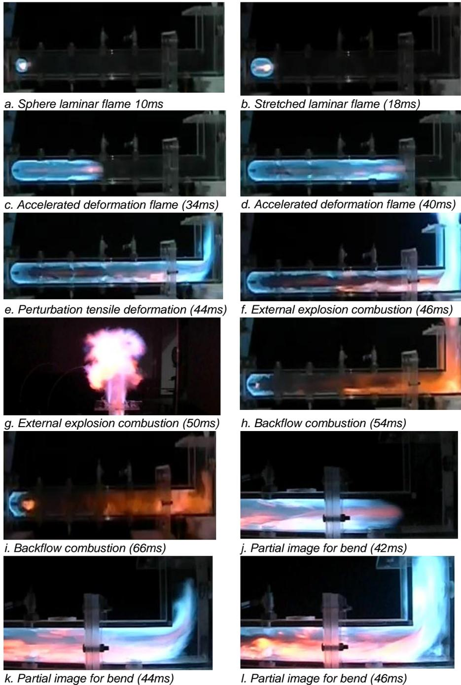
Figure 3: Flame propagation image
