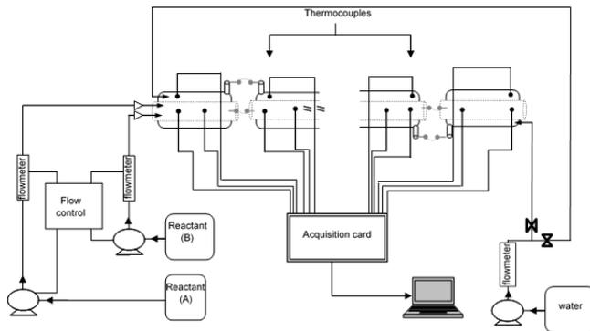
Figure 1: Experimental set-up of the tubular reactor.
