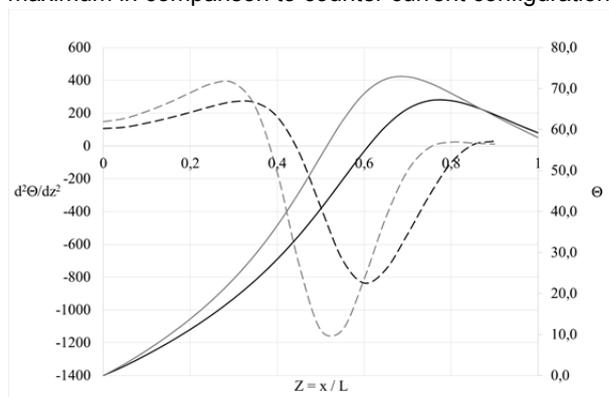
Figure 5: Second order derivative (dotted line, primary axis) of the profile of temperature (solid line, secondary axis) versus axial coordinate ( $Z=x/L$ ) for the case of co-current flow. In black co-current ; in grey counter current.
