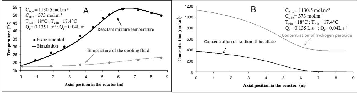
Figure 3:A: Reaction mixture and cooling fluid temperature profiles with co-current flow configuration.
