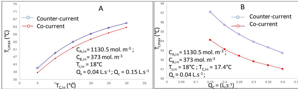
Figure 4: A: Effect of the inlet coolant temperature on the maximum reaction temperature.
