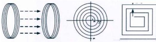
Figure 6: common magnetic coupling resonant coil structure
