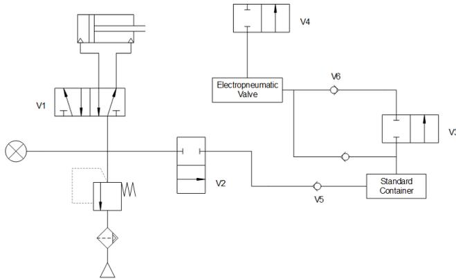
Figure 1: Schematic diagram of pneumatic circuit
