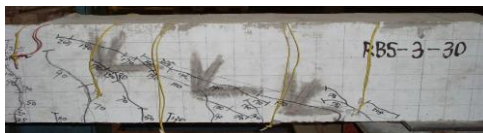
Figure 2: Oblique failure mode (E-surface)
