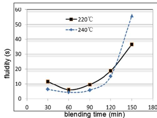
Figure 5: The Relational Graph of the Fluidity and Blending Temperature
