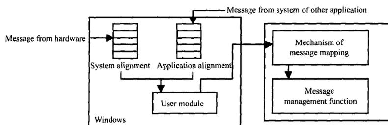
Figure 2: Message management mechanism for Windows
