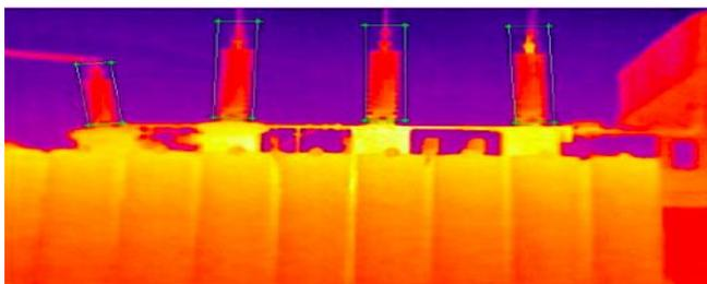
Figure 7: Infrared diagnosis of electrical equipment fault
