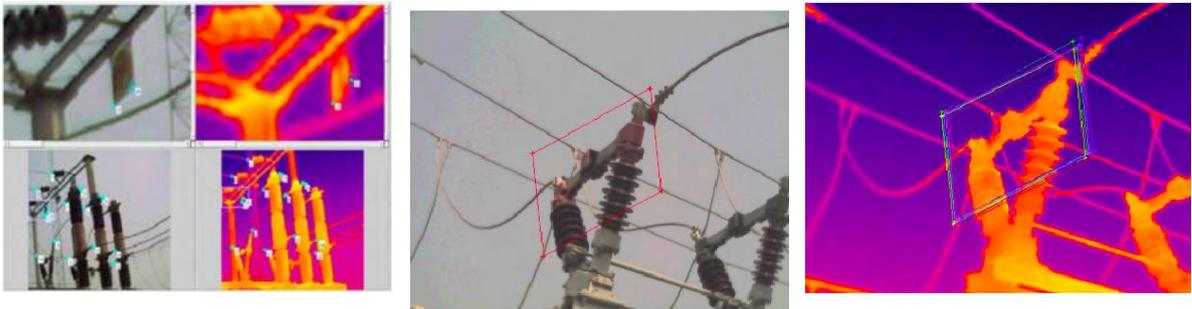
Figure 2: Corresponding points in infrared images and visible light target images
