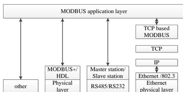
Figure 1: Modbus communication stack
