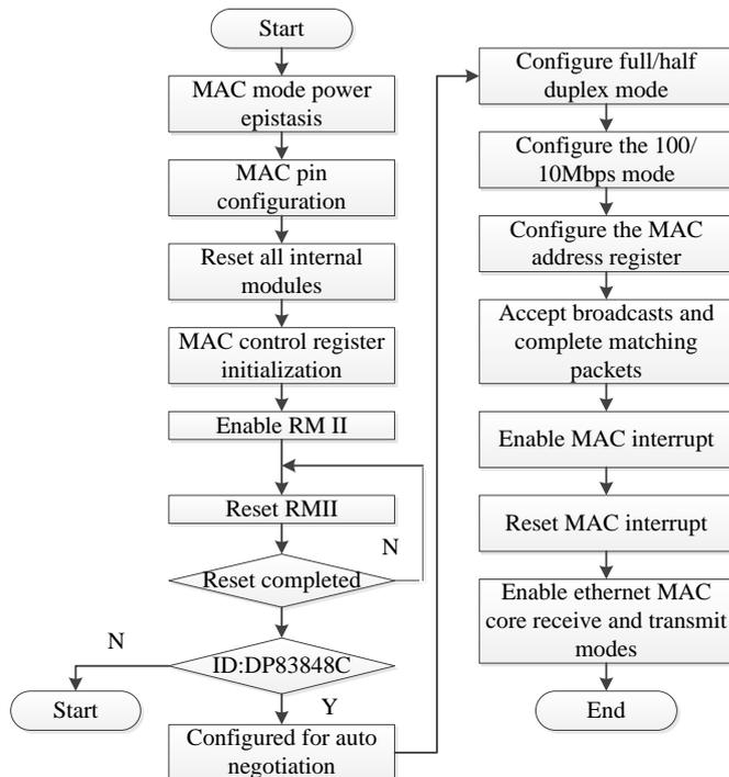
Figure 4: Ethernet software initialization program
