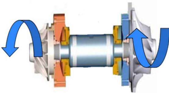
Figure 2: The internal structure of the expander.
