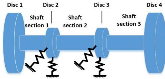
Figure 3: The mechanical model of turbo expander rotor.
