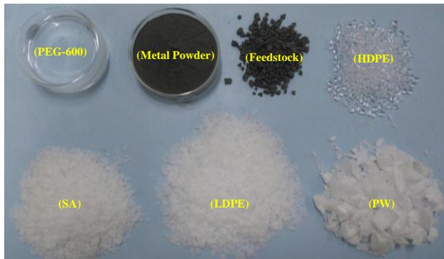
Figure 2: Basic materials for preparation of feedstock
