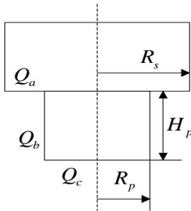
Figure 1: The stirring head shape
