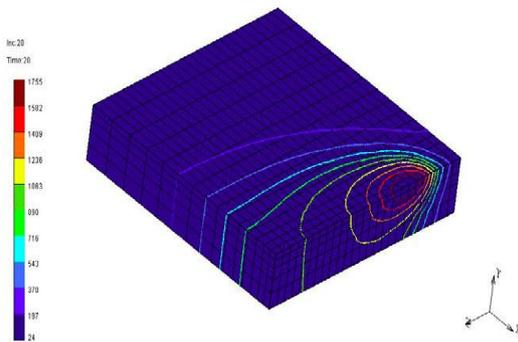
Figure 3: The welding temperature distribution at the same time obtained
