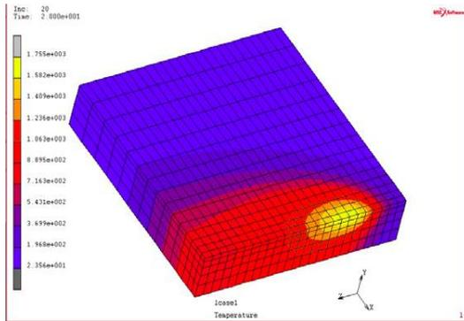
Figure 4: The plate welding isotherm distribution at a certain moment in the process
