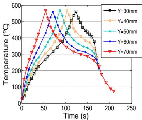
Figure 5: Nine weld center Y direction ( $Z=1.5\text{mm}$ ) temperature change curves of different points
