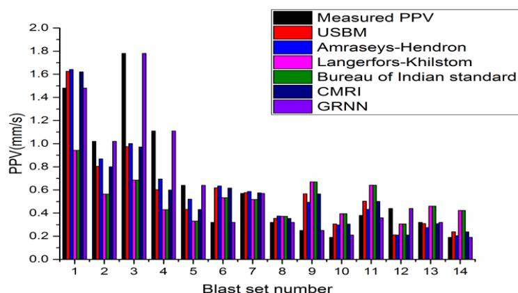
Figure 11: Comparison of measured and predicted PPV using different predictors
