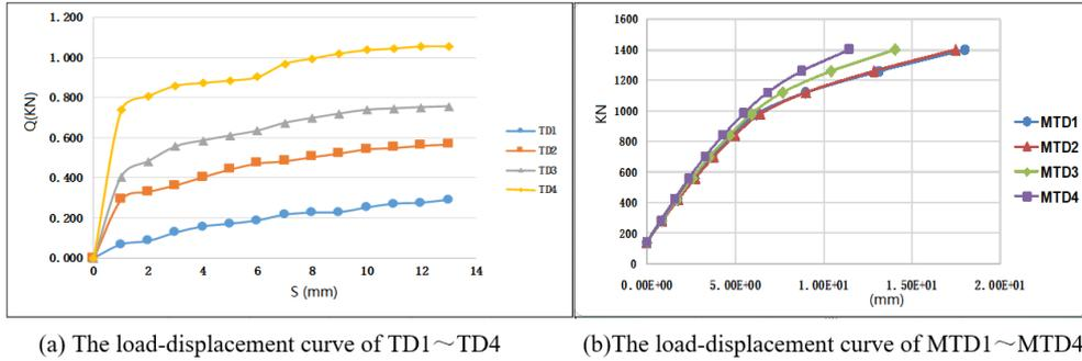
Figure 11: L-d curves in the model test and the simulation with different suspension diameters of the enlarging plate
