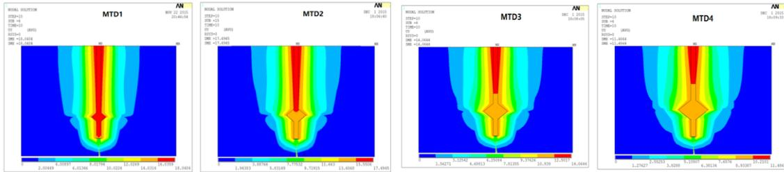
Figure 9: The Y-direction soil displacement of model piles with different suspension plate diameters
