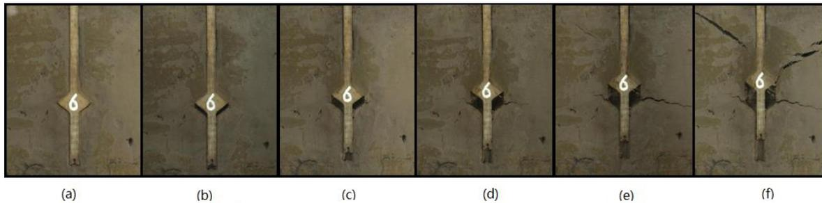
Figure 3: The whole process of soil destruction of Pile TD2
