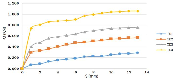
Figure 8: The contrastive S-Q curves of Model piles TD1, TD2, TD3, TD4
