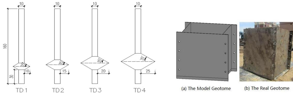
Figure 1: Design charts of the CEP pile with different diameters    Figure 2: The geotome
