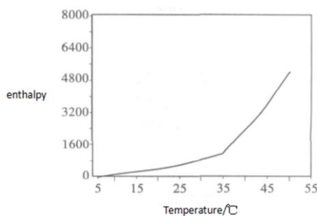
Figure 6: The change of enthalpy of paraffin wax with the change of temperature of ANSYS
