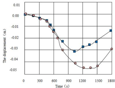
Figure 4: the horizontal displacement curve of the top end of the fire side
