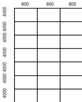
Figure 2: diagram of plane steel frame calculation
