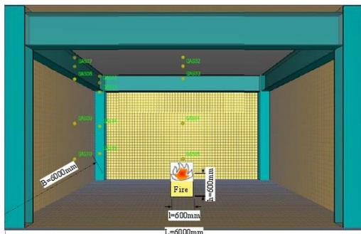
Figure 1: interior fire model of steel frame
