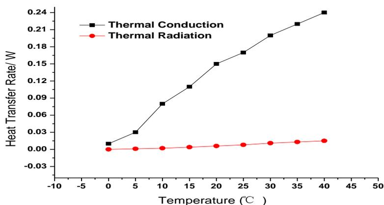
Figure 3: Curves of heat radiation and heat conduction on the thermal flow of a building sample
