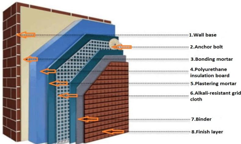
Figure 1: Schematic diagram of the structure of polyurethane thermal insulation composite exterior wall insulation system
