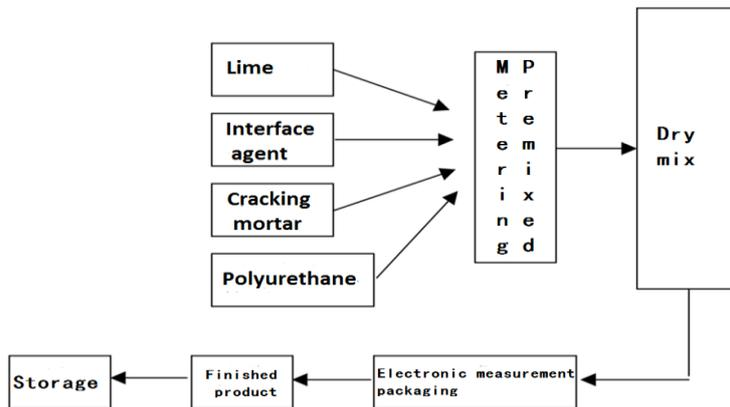
Figure 2: Process flow chart for the production of polymer dry powder mortar
