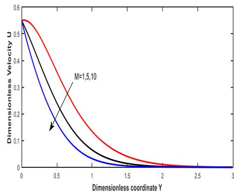
Figure 1b: Velocity profile for different magnetic parameter
