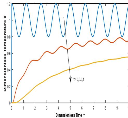
Figure 3b: Transient temperature at different points on the Y coordinate
