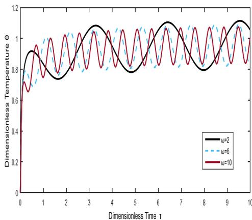
Figure 4a: Transient temperature for different values of temperature frequency
