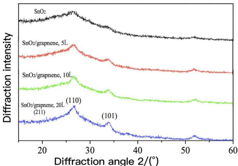
Figure 1: XRD spectra of tin oxide films doped with different layers of graphene (L-layer)
