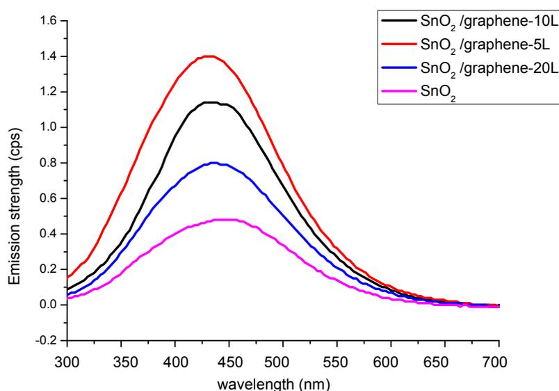
Figure 2: Photoluminescence spectra of tin oxide films with different layers of graphene doping concentration
