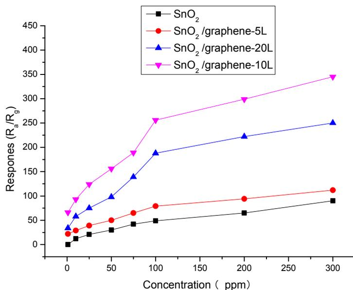
Figure 4: Responses of pure SnO<sub>2</sub> and SnO<sub>2</sub>/graphene nanocomposites to acetaldehyde with various concentrations at 120 °C
