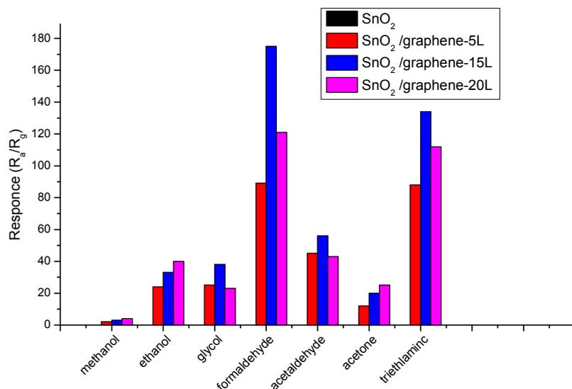
Figure 3: Sensor responses of pure SnO<sub>2</sub> and SnO<sub>2</sub>/graphene to 50 ppm of different gases at 120 °C
