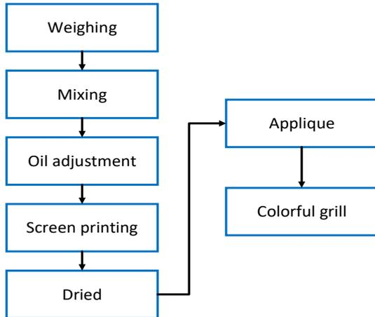
Figure 1: Color baking process flow chart
