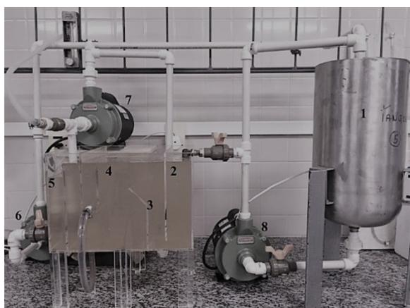
*Figure 1: Three dimensional scheme of pilot scale DAF system. Oily water storage tank (1); Flotation chamber (2); Second section where separation between treated water and oily foam formed (3); Oily foam collectors (4); Chamber of treated water collection (5); Return pump for treated water (6); Microbubble production pump (7); and oily water production pump and DAF chamber feed (8)*
