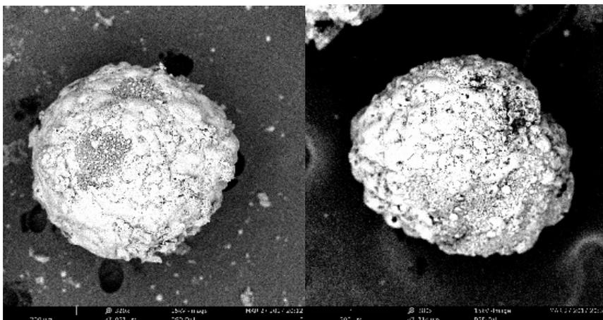
Figure 2: SEM of the microcarriers obtained for low voltage (14 kV, left) and high voltage (17 kV, right).
