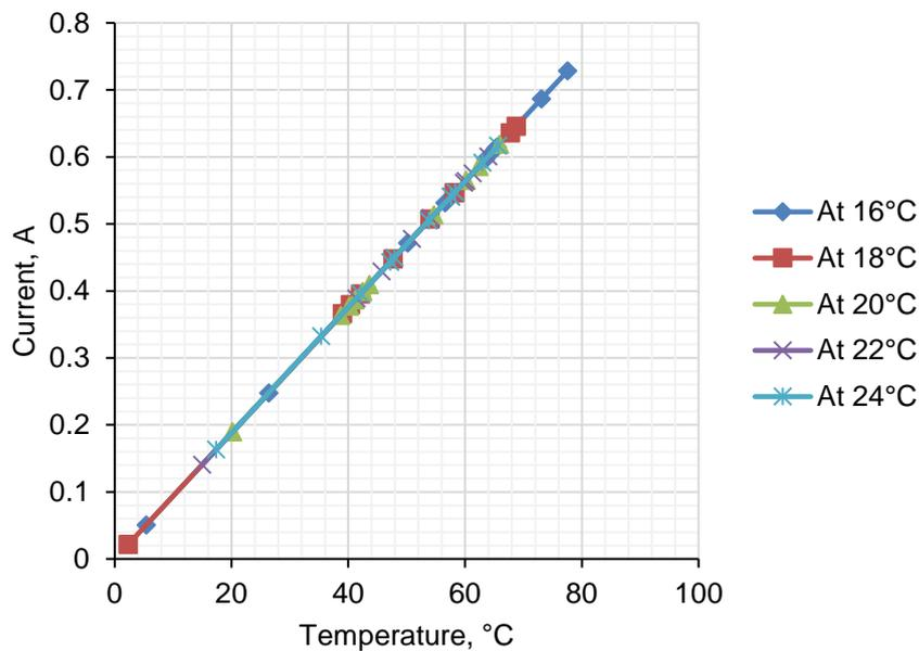
Figure 6: Output Current versus Temperature Different at different thermostat's temperature
