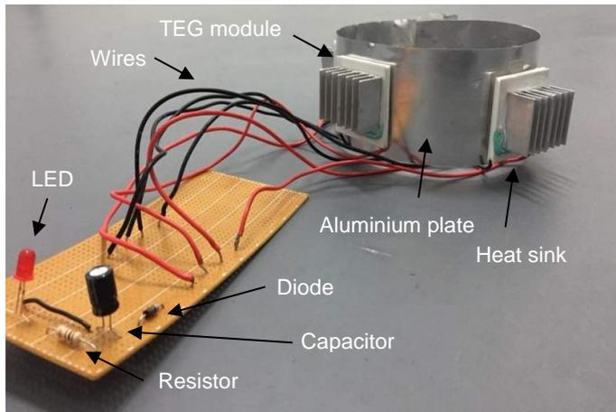
Figure 1: Prototype of TEG system attached at the air conditioning compressor.
