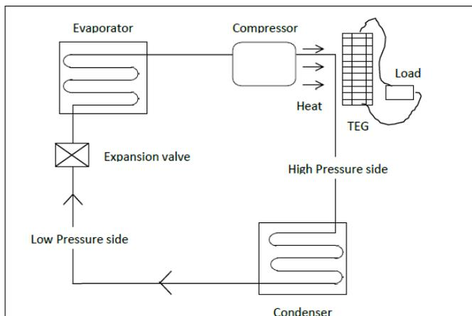
Figure 2: TEG system installed at the air conditioning compressor.
