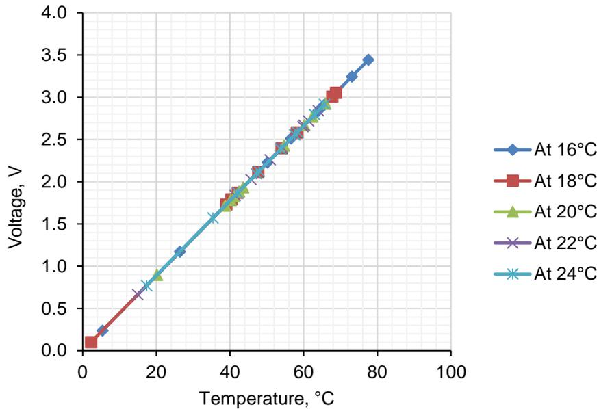
Figure 5: Output Voltage versus Temperature Difference at different thermostat's temperature setting
