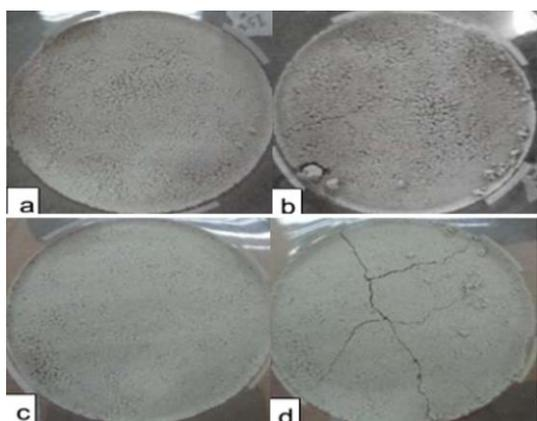
Figure 1: (a) Soil sample 1 before vibration process, (b) Soil sample 1 after vibration process with fracture, (c) Soil sample 2 before vibration process, and (d) Soil sample 2 after vibration process with fracture
