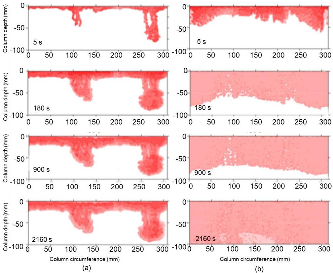
Figure 3: HSI plots of downward migration in fracture double-porosity soil (a) APL sample, (b) NAPL sample
