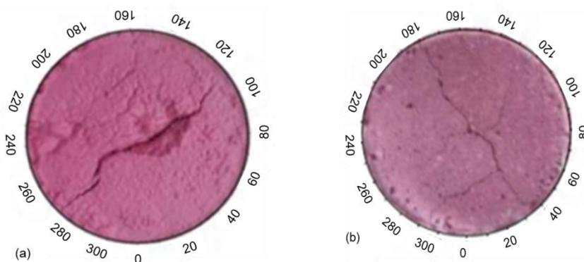
Figure 2: Migrated soil surface with measurement of actual column circumference zone (a) APL sample, (b) NAPL sample
