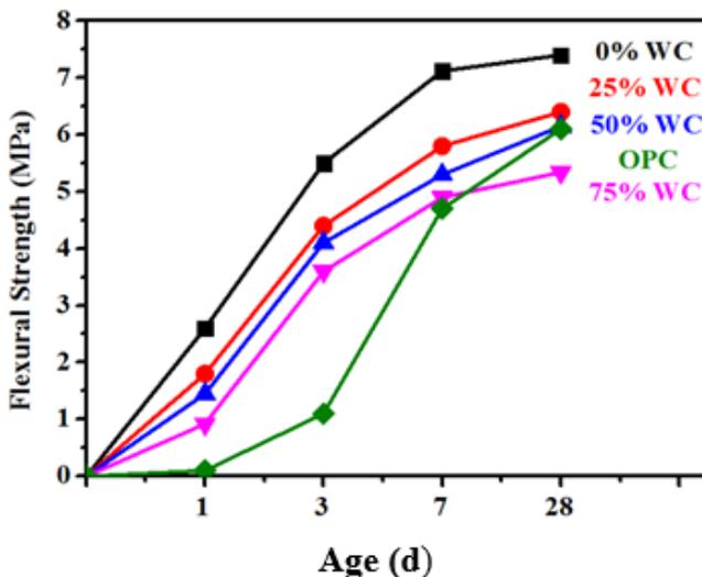
Figure 5: Flexural strength of mortar with various WC:GBFS
