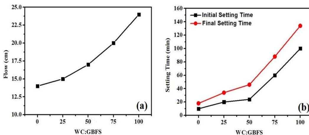
Figure 1: Effect of different ratios of WC: GBFS on (a) flow (b) setting time of alkali-activated mortars
