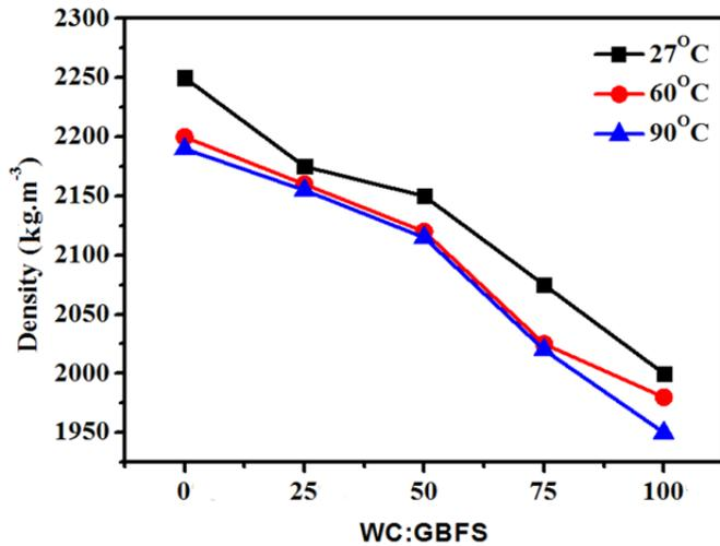
Figure 2: Effect of ceramic binder percentage on the density of alkali-activated.
