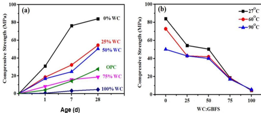
Figure 3: Development of compressive strength with various WC:GBFS (a) with age (b) with curing regime
