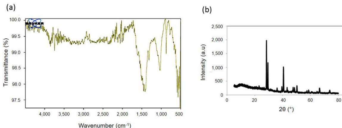
Figure 1: (a) FTIR spectra and (b) XRD diffractogram of water lettuce carbon
