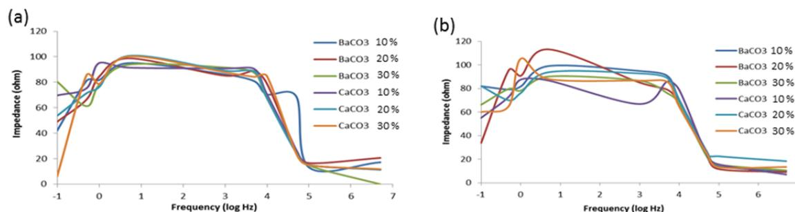
Figure 6: Impedance spectrogram of (a) asymmetric and (b) symmetric EC using 70 % WL carbon
