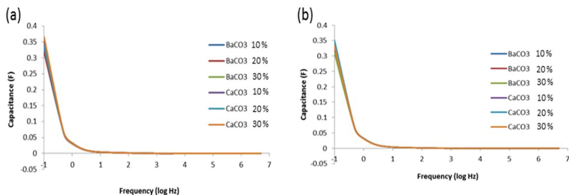
Figure 4: Capacitance plot of (a) asymmetric and (b) symmetrical EC with 70 % of WL carbon
