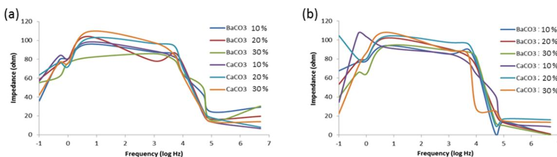
Figure 5: Impedance spectrogram of (a) asymmetric and (b) symmetric EC using 30 % of WL carbon
