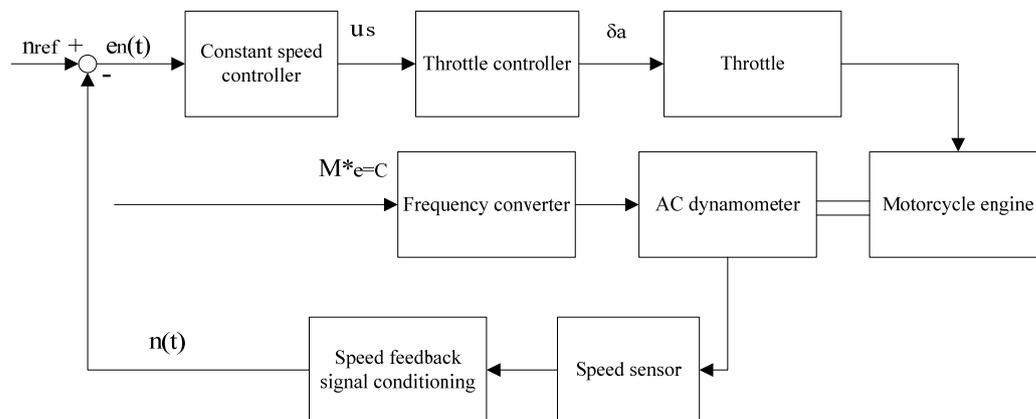
Figure 2: Control block diagram of load characteristics
