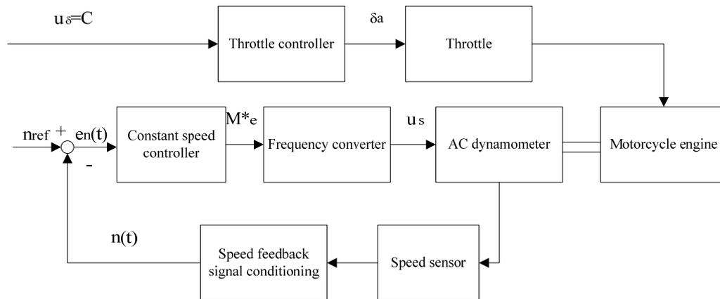
Figure 1: Control block diagram of speed characteristics
