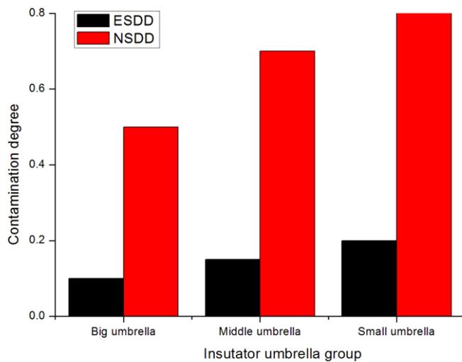
Figure 3: Distribution of fouling in different umbrella groups of composite insulators
