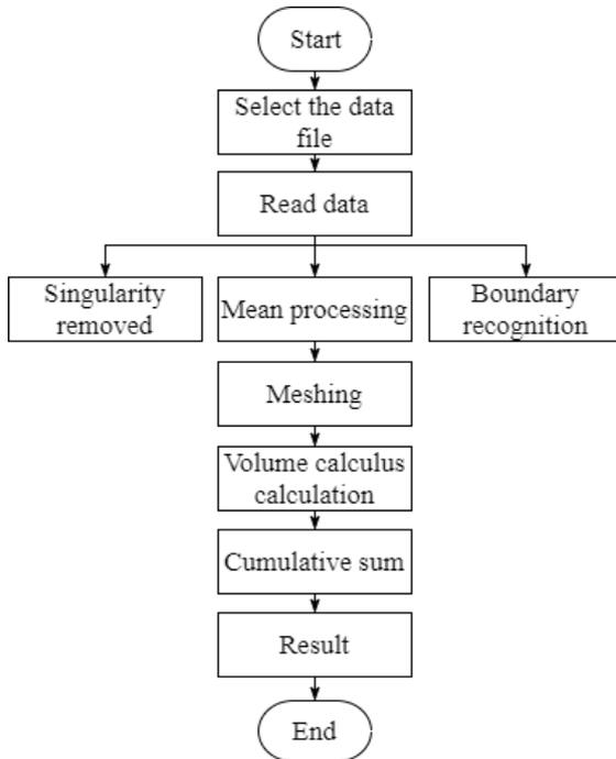
Figure 5: Flowchart of Volume Calculation
