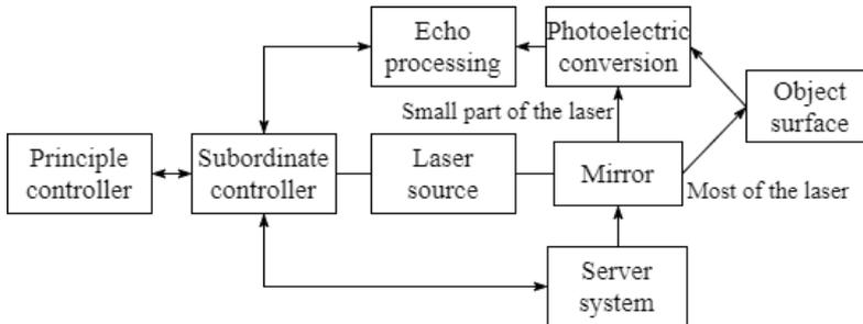
Figure 1: General Structure Block Diagram of 3D Laser Scanner
