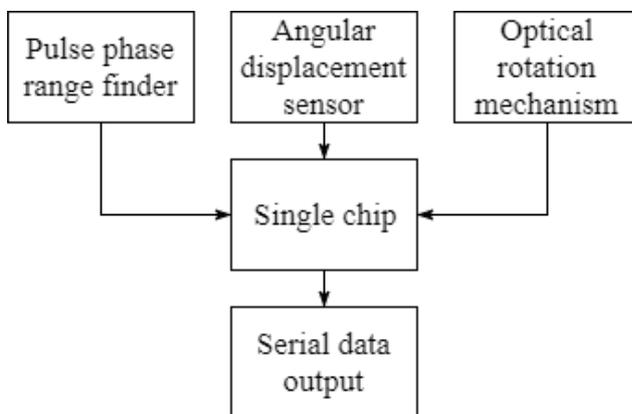
Figure 4: Schematic Diagram for Structure of Laser Scanner
