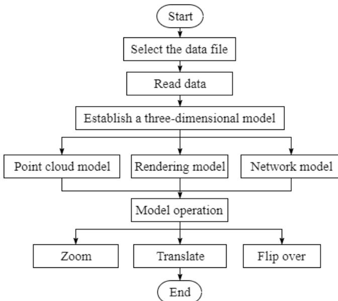
Figure 6: Model Reconstruction Flowchart
