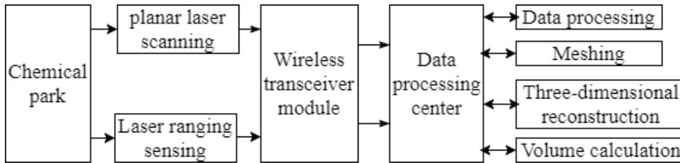
Figure 3: Block Diagram for System Hardware
