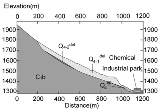
Figure 4: Cross-section of the talus slope
