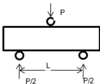
Figure 1: Schematic Diagram of Bending Test
