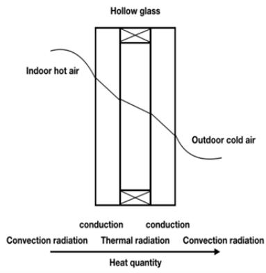
Figure 2: Heat lose channels of hollow glass
