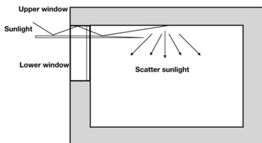
Figure 4: Illumination principle of lighting clapboard
