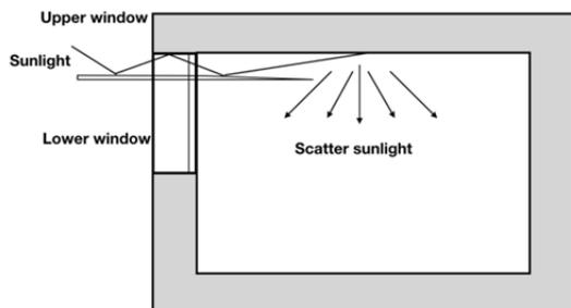
Figure 4: Illumination principle of lighting clapboard
