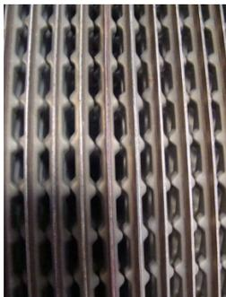
Figure 2: Experimental section of the corrugated plate heat exchanger
