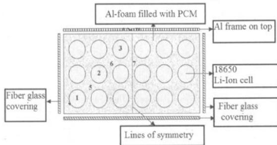
Figure 3: Battery Module of the Scooter
