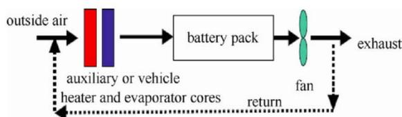
Figure 5: Air Cooling System Schematic Diagram
