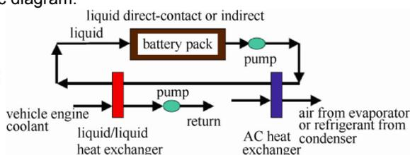
Figure 6: Liquid Cooling System Schematic Diagram
