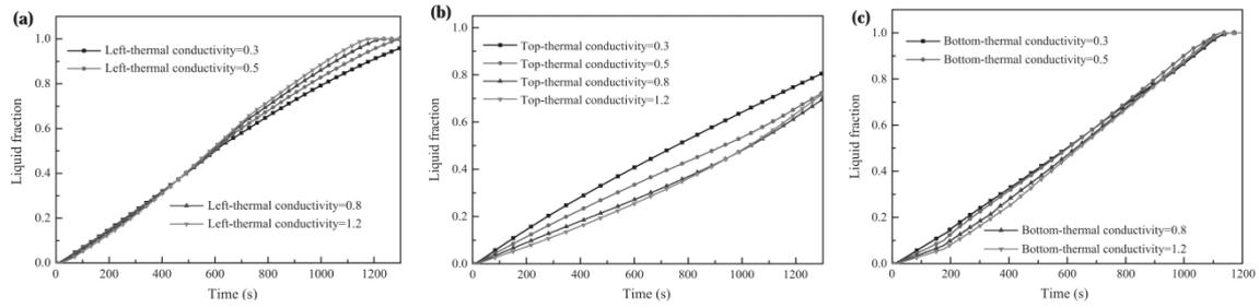
Figure 2: Effects of the Thermal Conductivity of PCM on the Phase Change Process. Heat flux was Applied to the Left Wall (a), the Top Wall (b) and the Bottom Wall (c)
