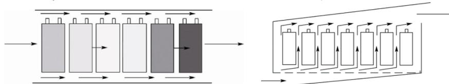
Figure 4: Serial Airflow Scheme and Parallel Airflow Scheme
