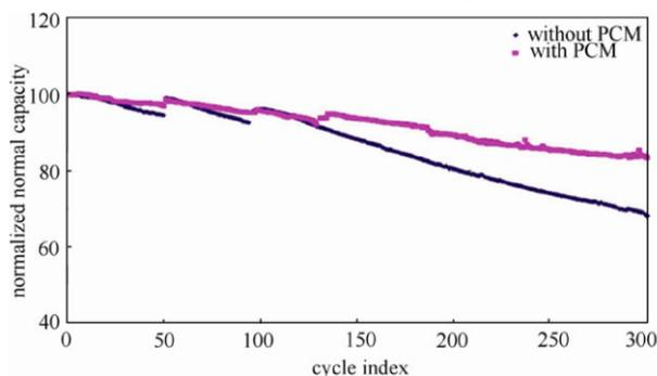
Figure 7: The Capacity Fade Testing of Battery Modules with/without PCM.
