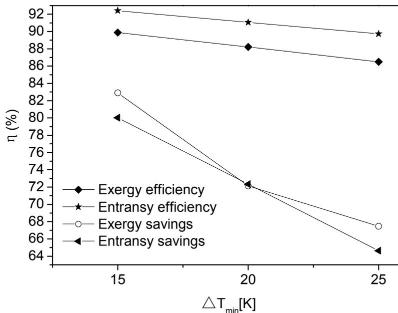
Figure 3: The efficiency of different  $\Delta T_{\min}$
