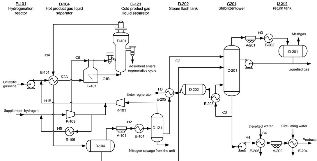
Figure 1: The process flowsheet of S-zorb unit
