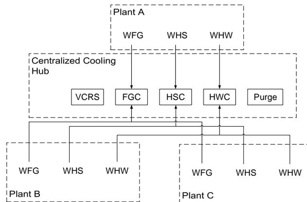
Figure 1: Waste heat and refrigeration system superstructure representation for proposed network (HSC = Hot steam ARS, HWC = Hot water ARS, FGC = Flue gas ARS)
