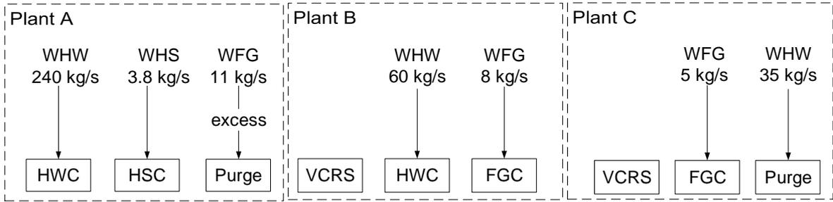
Figure 2: Waste heat and refrigeration system superstructure representation without centralized cooling hub
