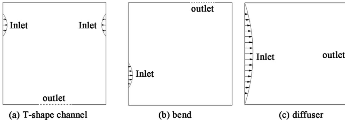
Figure 1: Computation domains and boundary conditions for a T-shape channel, a bend and a diffuser
