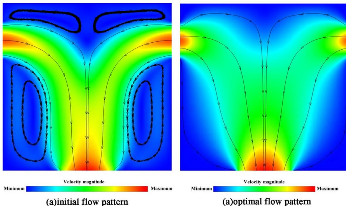
Figure 2: Comparison of initial and optimal flow patterns in initial computational domain when  $Re=50$
