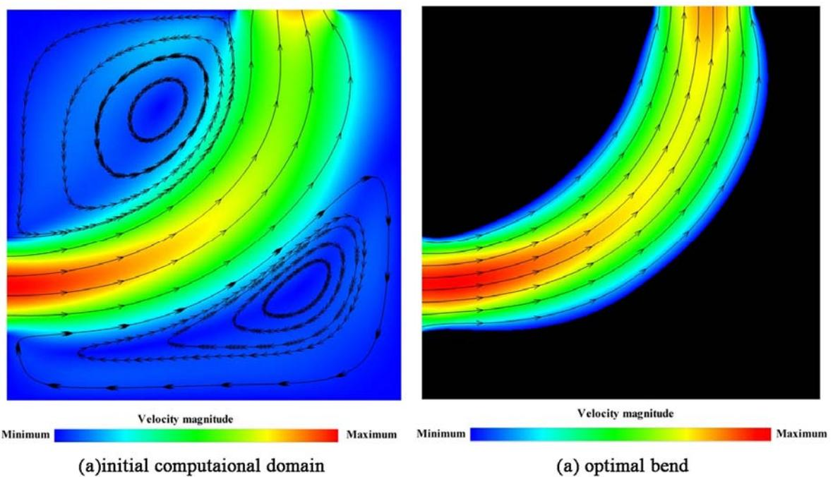
Figure 4: Comparison of the flow patterns in initial computational domain and optimal bend when  $Re=75$
