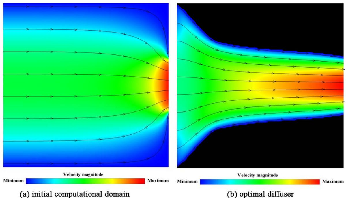
Figure 5: Comparison of the flow patterns in initial computational domain and optimal diffuser when  $Re=54$
