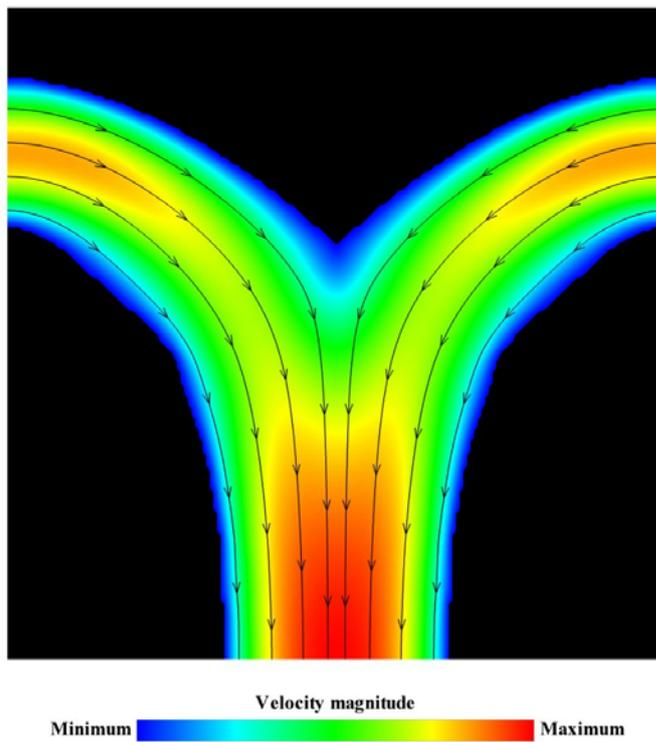
Figure 3: Optimal T-shape channel with flow field and streamlines
