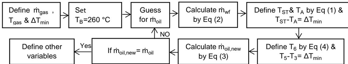
Figure 3: Trial and error algorithm for solving the ORC's thermodynamic equations
