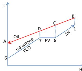
Figure 2: T-H diagram of the heat recovery
