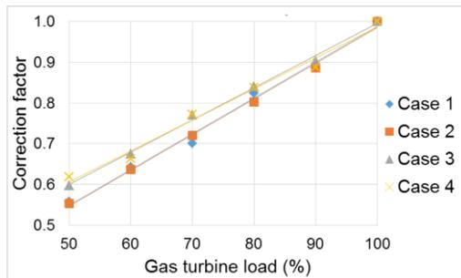
c) Correction factor of ORC's power in  $\Delta T_{min} = 20$  °C and different turbine load
