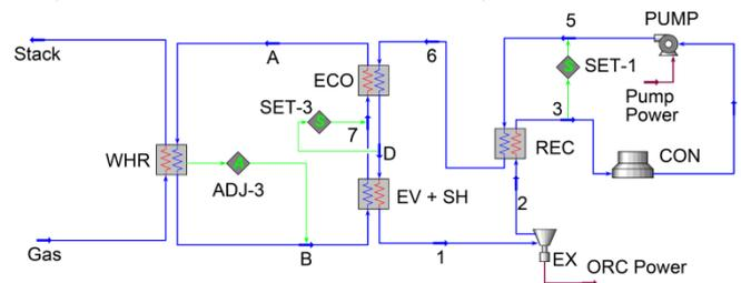
Figure 4: Simulation's flow diagram of Organic Rankine cycle
