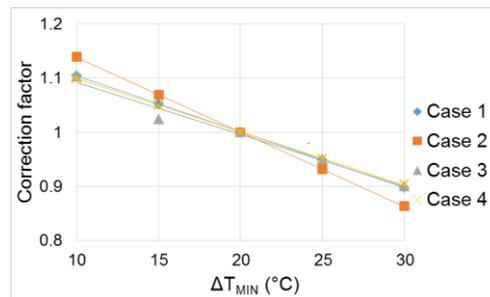
d) Correction factor of ORC's power in turbine load = 100 % and different  $\Delta T_{min}$ Figure 5: Investigating the influence of turbine load and  $\Delta T_{min}$  on the ORC's power
